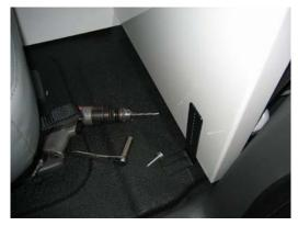
Attach front partition to vehicle using 6" L-mounting bracket. Bolt bracket to partition using <sup>1</sup>/4" x <sup>3</sup>/4" carriage bolts and nuts. Bolt "L" mounting bracket to vehicle using <sup>1</sup>/4" x 1" Lag bolts. Pre-drill w/ 3/16" hole
